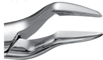
32 Parmly Alveolar Forceps Upper Canines, Premolars & Molars; Universal. Sharp edged beaks for breaking the alveolar process and trimming it after extraction. F32
